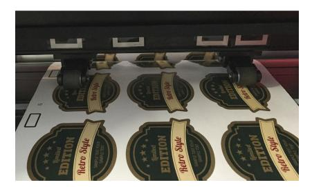
Then close the black clamp lever on the cutting head and complete the inserting the foil thereby.
