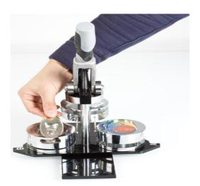
• Move the right side of the rotary disc backwards below the upper mold.
