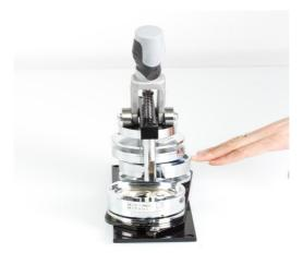
• Now press the parts of the upper shell with medium pressure. The upper parts of the badge should be pinned in the upper mold.
