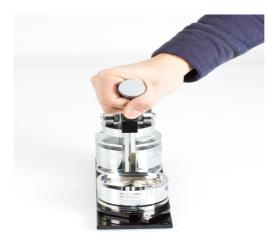
Notice: If the mechanical stops moved a little bit after long term use, they can be adjusted with a cross-head screwdriver.
