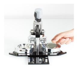
• Place the punched motive on top of the upper shell into the right tool.
