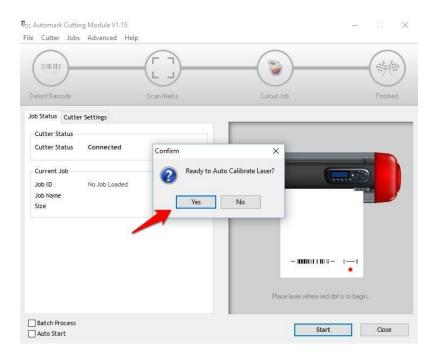
• The cutter will now automatically perform the calibration and report the correct laser offset for your device, which you need to confirm by clicking on "OK".
