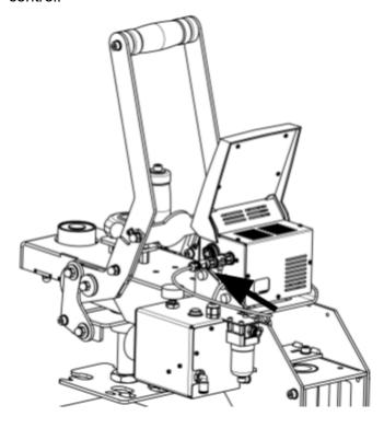
Position the Secabo SH7 Softheat heating membrane in front of the connection flange below the press lever on the Secabo TS7 Smart at an angle and thread the 4 external screw heads into the keyhole millings on the flange plate. The entire process is performed according to the same scheme as the installation of the standard HP7 heat plate.
