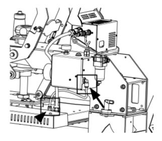
Now attach the compressed air hose (6 mm) to the connection for the external compressed air supply. Do this by using the Pneufit on the pressure reducer. In the last step, connect the other end to your external compressed air supply, whereat the input pressure must not exceed **maximum 8 bar. Only use the supplied connection material to prevent material** damage to the machine.
