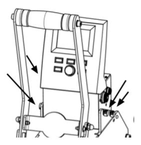
Next, attach the Secabo SH7 Softheat pneumatic control to the free-standing threaded pins, as viewed from the front right. Fix the pneumatic control to the threaded pins using the two previously removed knurled nuts. Also tighten the knurled nuts on the left side again.
