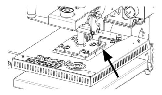
Plug the large 5-pin plug of the Secabo SH7 Softheat heating membrane into the matching socket on the outer right side of the **HPC01** Controller.
