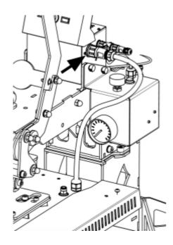
Next, connect the Secabo SH7 Softheat heating membrane to the Secabo SH7 Softheat pneumatic control using the compressed air hose (8 mm) included in the scope of delivery. To do this, you have to connect the compressed air hose to both the Secabo SH7 Softheat heating membrane and the Secabo SH7 Softheat pneumatic control using the provided pneufits.
