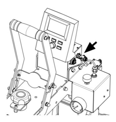
Now connect the cable harness of the Secabo TS7 Smart with the small 6-pin plug, which comes from the electromagnet, to the adapter of the Secabo SH7 Softheat pneumatic control.
