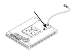
• Silicone mat of the heating membrane with embedded wires.
