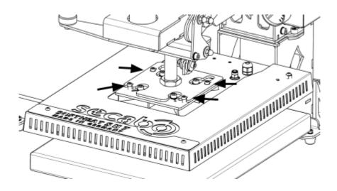
Carefully tighten the screws using the included Allen key (SW5). Attention: As long as the screws are not properly tightened, the heat plate may fall down! Risk of injury!
