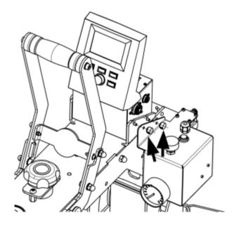
Connect the cable harness of the Secabo SH7 Softheat pneumatic control to the small socket of the HPC01 controller.
