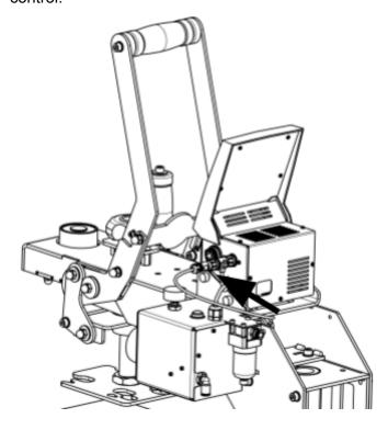
Position the Secabo SH7 Softheat heating membrane in front of the connection flange below the press lever on the Secabo TS7 Smart at an angle and thread the 4 external screw
