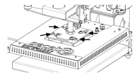
Carefully tighten the screws using the included Allen key (SW5). Attention: As long as the screws are not properly tightened, the heat plate may fall down! Risk of injury!
